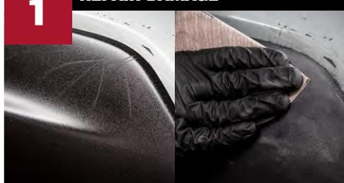
If extensive damage is present, refer to **Plastic Repair Standard Operating Procedure** first.
