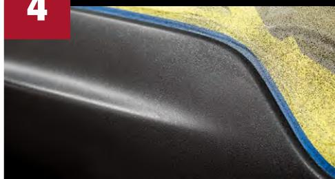
Apply **Bumper Coater™** or **Trim Black** as a wet bed over the extended repair area. Apply **Texture Coating** in light mist coats 12" - 24" from surface.
