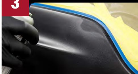
Sand any shallow scratches or scuffs until smooth. Blow off and wipe with a tack rag. Mask the area to be sprayed.
